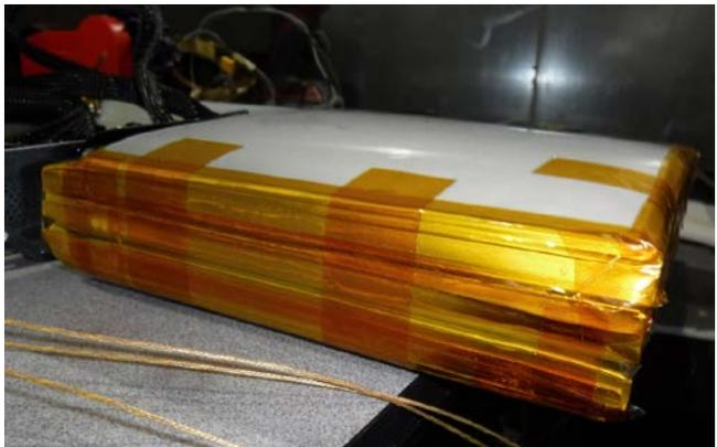
Fig. E7 – Internal cell group (view from cells facing the rear of module)
