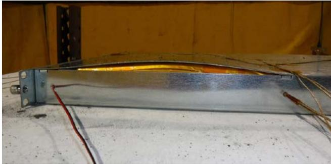
Fig. E3 – Measured expansion of 1cm.
