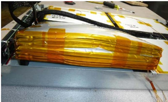
Fig. E5 – Internal cell group (view from cells facing the left side of module)
