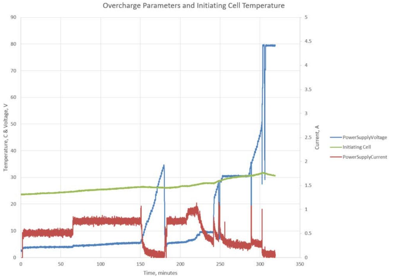
Fig D1 – Charging Voltage & Current, Initiating Cell Temperature
