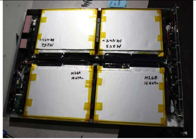
Fig. B3 – 8S/1P cell package (referred to as Module 2 internally – Natron)
