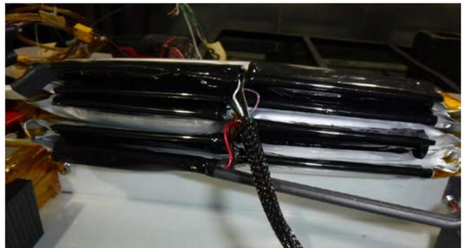
Fig. E6 – Internal cell group (view from cells facing the front of module)
