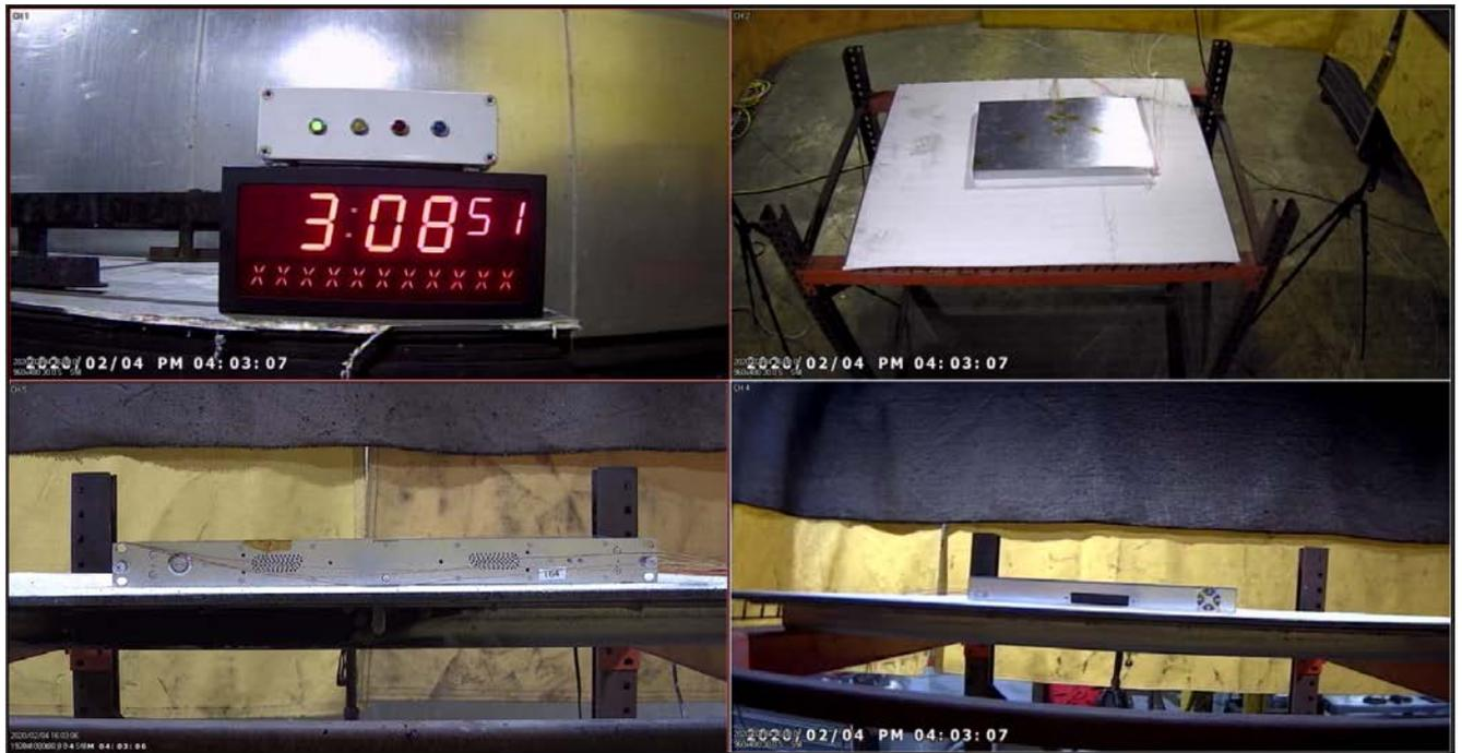
Fig. E1 - Initial Observation of the expansion of the initiating cell causing the enclosure to deform.
